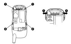
Release the front panel by moving the retention lugs
